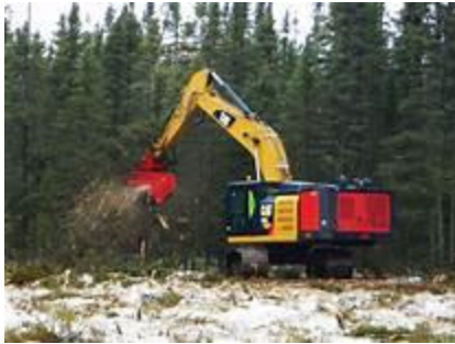
Excavator mounted forestry/mulching attachment
