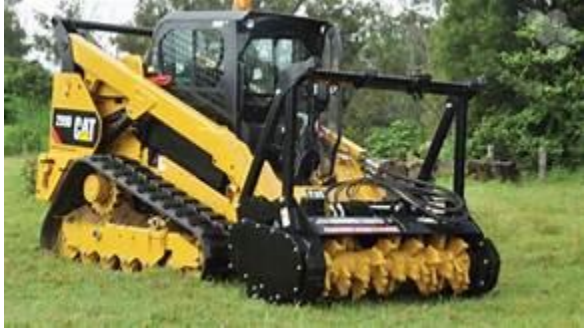
Skid steer loader mounted forestry/mulching attachment
